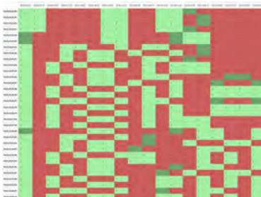
Figure 3: Coverage Map showing t -tuple coverage per parameter selection
