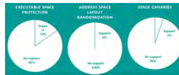
Figure 1: Availability of assorted security features in embedded systems without standard operating system. ("Ghost in the Machine: Challenges in Embedded Binary Security", Wetzels, Usenix Enigma, 2017)
