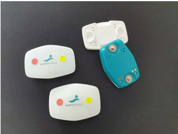
The first prototypes of the new HRV sensor generation © HeartBalance Innovations GmbH 2019
