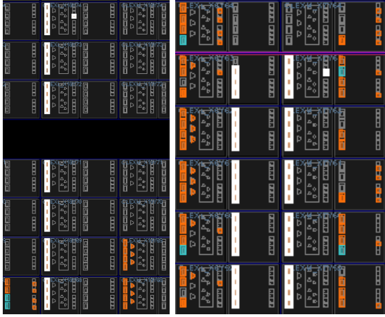
Fig. 5. Area covered by 27-bit RO (left) and 19-bit TERO (right)
