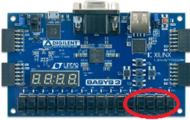
Figure 2: Basys3 FPGA development board with marked pushbuttons.
