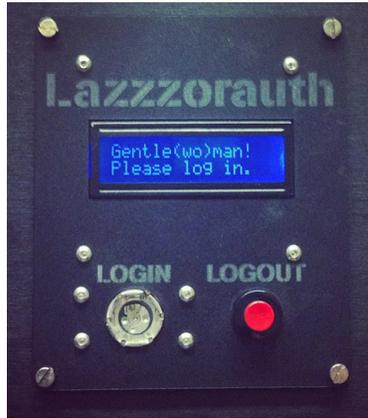
**Fig. 1.** A possible scenario: The current authorization for the laser cutter at Metalab Vienna, Austria uses iButtons against a central authorization database and a display. Wi-Fi presence information can simply be displayed to the screen if necessary.
